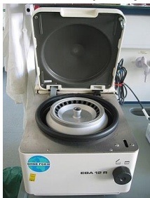
Obr. 46 centrifuga EBA 12 R
